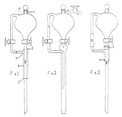
sists of a dropping funnel whose tube B passes through and is sealed to the tube A at E. The tube C with a glass stop-cock at D is fused into openings in the upper part of A at F and in the upper part of the funnel at K. The funnel is made with air vent in the stopper.
